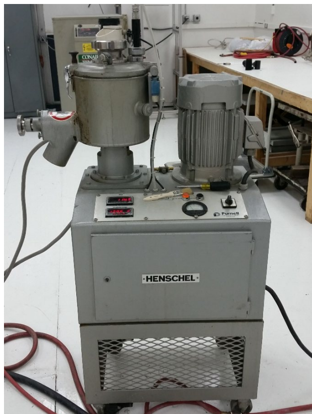
Fig. 1. Henschel mixer (left) and interior of mixer (right) with remnants of blended SRM 2859 ingredients. A water heater (not shown) maintains mixer jacket temperature.
