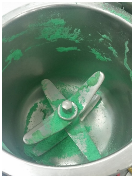
Fig. 1. Henschel mixer (left) and interior of mixer (right) with remnants of blended SRM 2859 ingredients. A water heater (not shown) maintains mixer jacket temperature.
