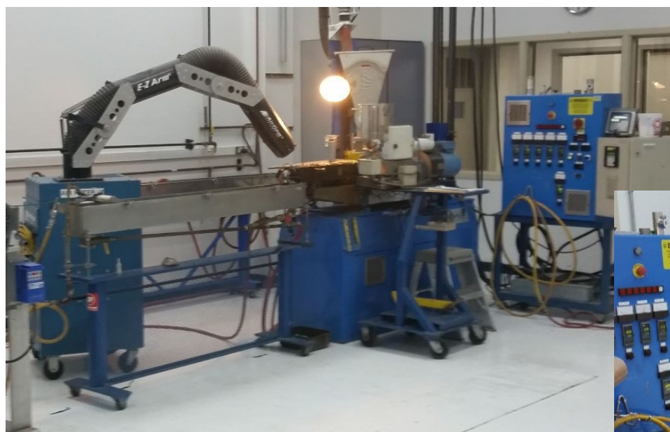
Fig. 2. Twin-screw extruder (center above) with controls to its right and water trough to its left. Arm above the trough is a fume extractor pointed at extruder exit die. Powder feeder on balance (right) dispensing powder for SRM 2861 into extruder.
