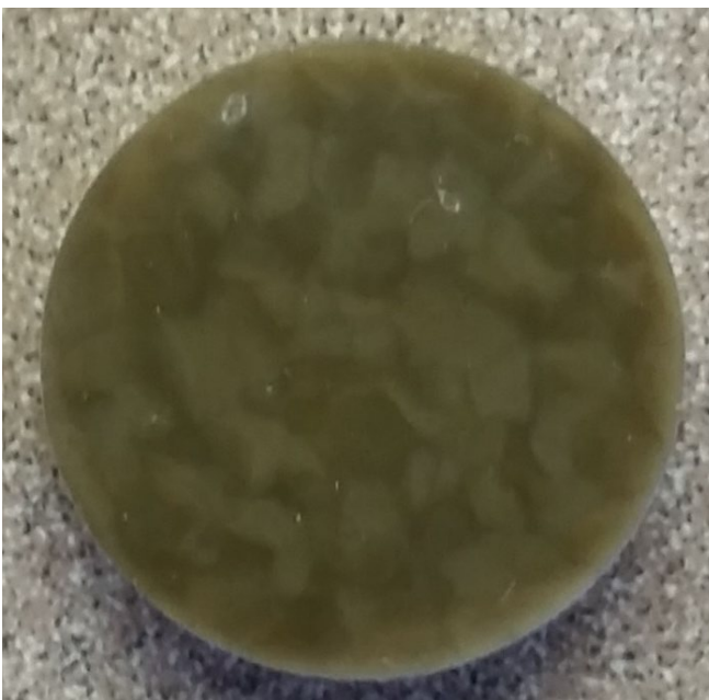
Fig. 6. Melt-pressed disk made from pellets of SRM 2861 heated to 175 °C for 1.5 h. Darker regions are outer surfaces of individual pellets.
