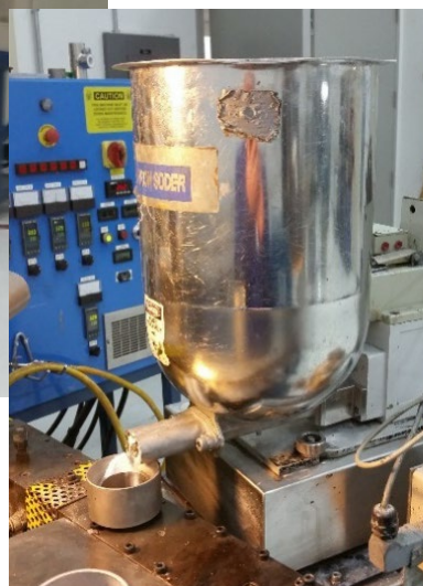
Fig. 2. Twin-screw extruder (center above) with controls to its right and water trough to its left. Arm above the trough is a fume extractor pointed at extruder exit die. Powder feeder on balance (right) dispensing powder for SRM 2861 into extruder.
