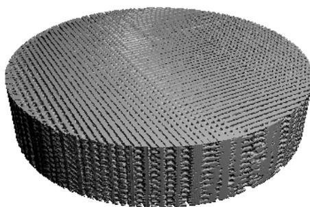
Figure 1. X-Ray Microcomputed Tomograph of Reference Scaffold RM 8396.
