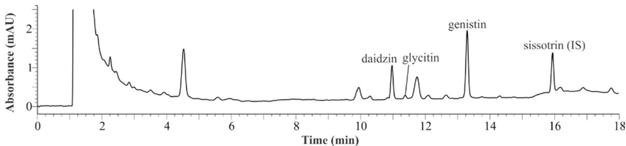
Figure 2. Chromatogram showing separation and detection of isoflavones in SRM 3237 using LC/absorbance. For this method, an Ascentis Express RP-Amide column (150 mm × 4.6 mm, 2.7 μm particle size; Supelco, Bellefonte, PA, USA) was held at 35 °C. The separation was performed using a gradient consisting of 5 mmol/L ammonium acetate in water and acetonitrile. Absorbance detection was utilized at 254 nm.
