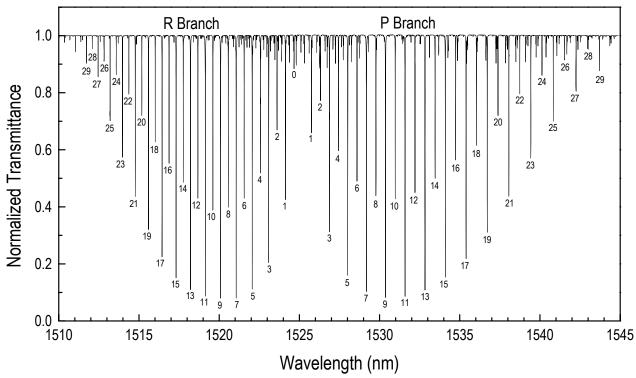
Figure 1. Normalized spectrum of SRM 2517a obtained by scanning a tunable diode laser and measuring the laser power transmitted through a SRM unit. The SRM contains a 5 cm long absorption cell filled with acetylene  $^{12}C_2H_2$  to a pressure of 6.7 kPa (50 Torr). A file containing these data can be downloaded from the data file link on this web page: <a href="http://ts.nist.gov/srmcertificate/?srm=2517a">http://ts.nist.gov/srmcertificate/?srm=2517a</a>.
