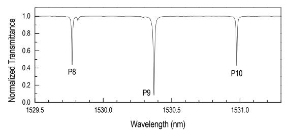
Figure 3. Spectrum of the P8, P9, and P10 lines from Figure 1 obtained by scanning a tunable diode laser.
