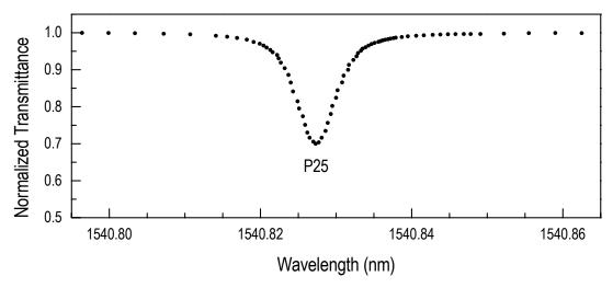
Figure 2. Spectrum of line P25 from Figure 1 obtained by scanning a tunable diode laser.
