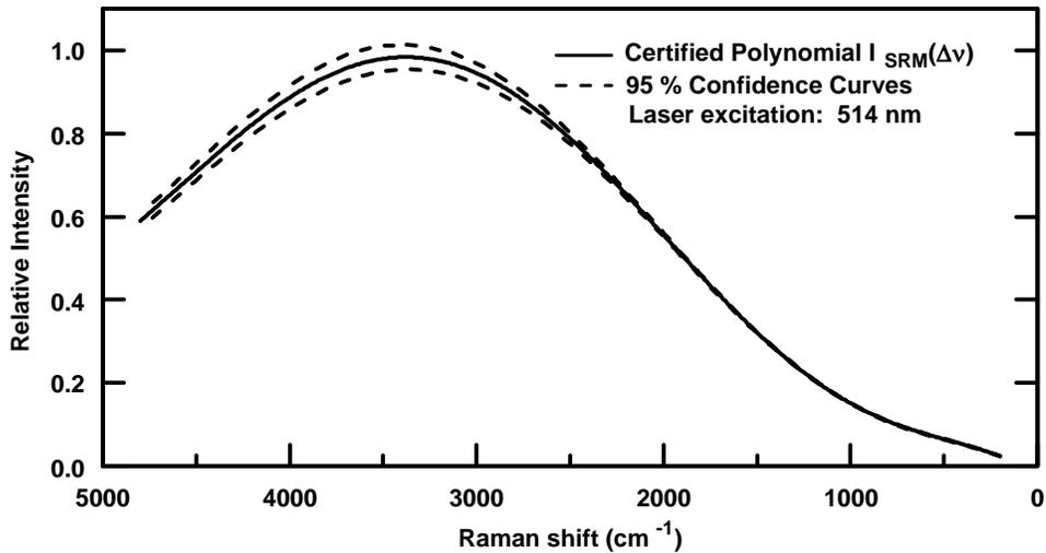
Figure 3: Sixth-order certified polynomial for SRM 2243. The x-axis is expressed in Raman shift ( $\text{cm}^{-1}$ ) relative to 514.5 nm ( $19\,435.18\ \text{cm}^{-1}$ ). The y-axis is on a relative scale and normalized to unity with the dimensions of photons  $\text{s}^{-1}\text{cm}^{-2}(\text{cm}^{-1})^{-1}$ . Dashed lines indicate 95 % confidence curves.
