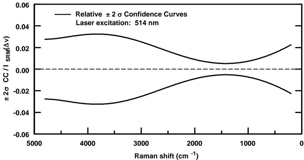
Figure 4. Relative  $\pm 2\sigma$  confidence curves describing the luminescence spectrum of SRM 2243. The two solid black curves represent for SRM 2243 at room temperature, respectively, the quotient  $\pm 2\sigma\ \text{CC} / I_{\text{SRM}}(\Delta\nu)$ . The certified polynomial is valid over the temperature range of 20 °C to 25 °C. The x-axis is Raman shift (relative to 514.5 nm,  $19\,435.18\ \text{cm}^{-1}$  laser excitation).
