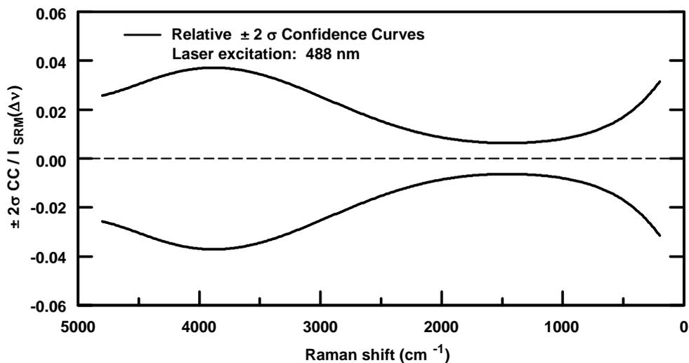
Figure 2. Relative  $\pm 2\sigma$  confidence curves describing the luminescence spectrum of SRM 2243. The two solid black curves represent for SRM 2243 at room temperature, respectively, the quotient  $\pm 2\sigma$  CC / I<sub>SRM</sub>(Δν). The certified polynomial is valid over the temperature range of 20 °C to 25 °C. The x-axis is Raman shift (relative to 488 nm, 20 492.35 cm<sup>-1</sup> laser excitation).
