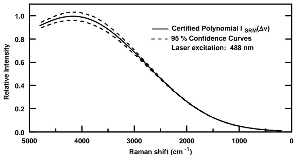
Figure 1. Sixth-order certified polynomial for SRM 2243 when excited at 488 nm. The x-axis is expressed in Raman shift (cm<sup>-1</sup>) relative to 488 nm (20 492.35 cm<sup>-1</sup>). The y-axis is on a relative scale and normalized to unity with the dimensions of photons s<sup>-1</sup>cm<sup>-2</sup>(cm<sup>-1</sup>)<sup>-1</sup>. Dashed lines indicate 95 % confidence curves.
