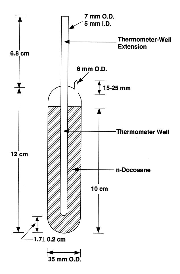
Figure 1. Cross-sectional drawing of the n-docosane triple-point cell.
