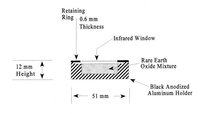
Figure 1. Cross-Section of SRM 1920a Holder
