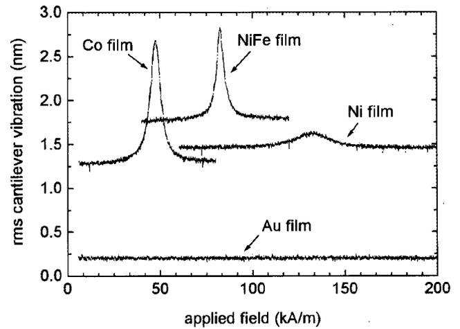
FIG. 3. Cantilever vibration vs applied field showing microwave absorption in Co, NiFe, Ni, and Au thin film samples.
