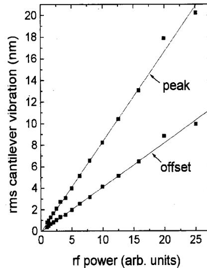
FIG. 5. Lorentzian peak and offset cantilever vibration vs input power for a 30 nm Co film (derived from the data in Fig. 4).
