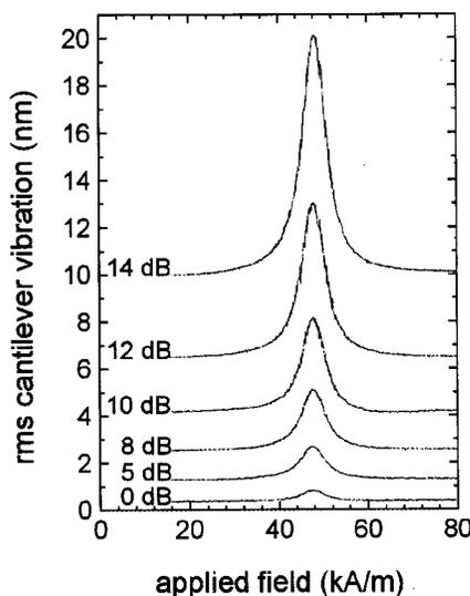
FIG. 4. Cantilever vibration vs applied field for a 30 nm Co film at different relative input microwave power levels.
