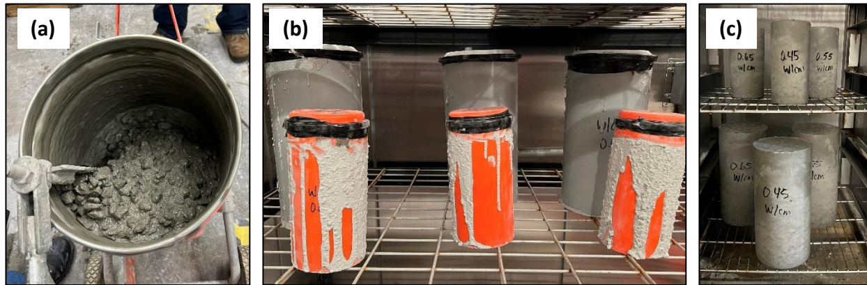
Figure 18. Mixing and curing process used for specimens to meet Goal 2 of study: (a) mixing concrete in bucket mixer; (b) initial 24 hour curing in sealed containers in temperature-controlled chamber; (c) room temperature, 100 % relative humidity curing chamber
