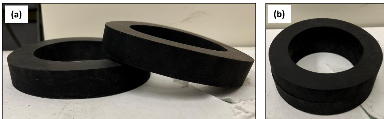
Figure 9. Machined neoprene inserts: (a) side view of two machined inserts; (b) two inserts stacked for testing
