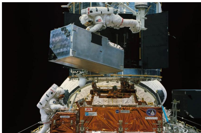
Figure 3: Corrective Optics prior to its installation into the Hubble Space Telescope. Image Credit NASA (public domain) [26].
