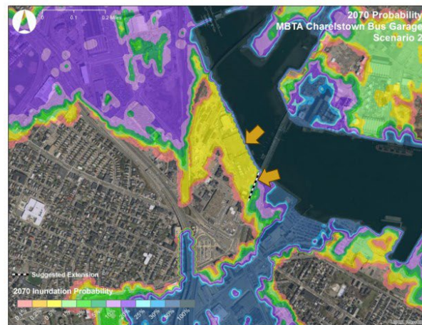
Figure 4. 2070 flood probabilities in the vicinity of the Charlestown MBTA Bus Depot with proposed resiliency design, including additional flood wall along Alford Street, in place.
