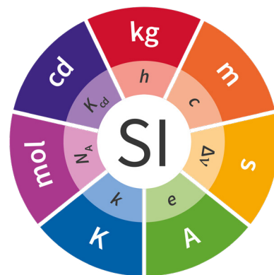
Figure 13. SI logo with seven defining constants and seven base units 9 . Credit: BIPM
