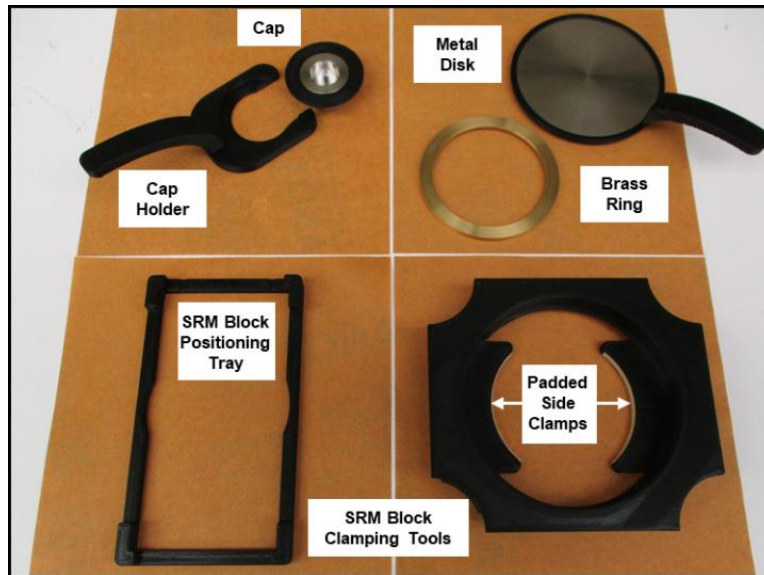
Figure 12. Components used in the SRM block seating process, including a non-magnetic cap to cover the indenter tip, a protective ring and disk assembly to safeguard the SRM block, and a positioning tray used with the clamping tool to align the block on the testing frame's anvil.
