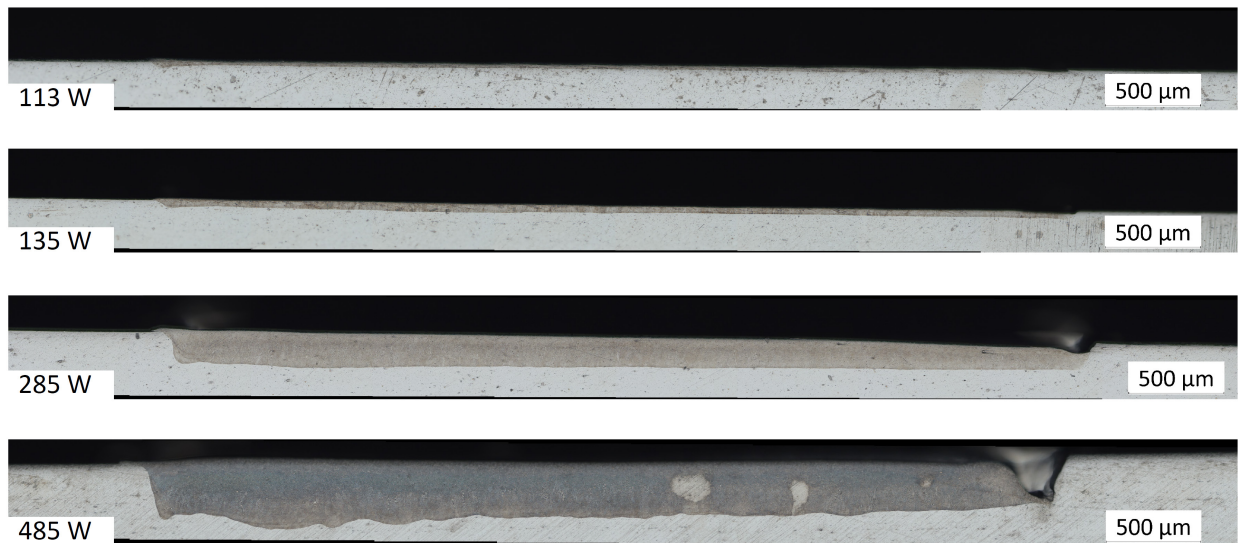
Fig. 9. Lengthwise cross-sections of samples at different laser power levels. (FIGURE WIDTH: 2 COLUMNS)
