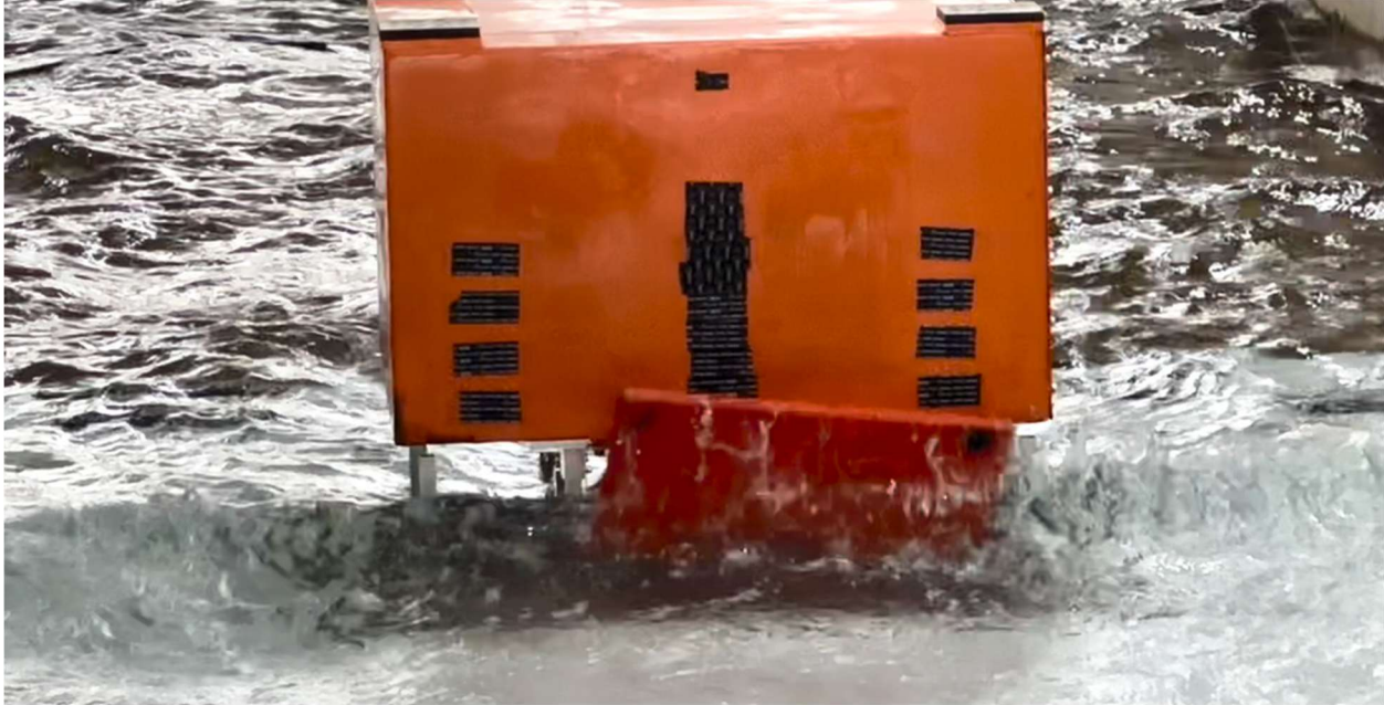
Figure 6. Plate-like debris in laboratory wave-current flow flipping vertically and impacting an elevated structure. These types of loads were found to consistently have the largest magnitudes when compared to other debris and load types.
