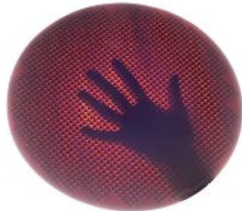
Fig. 18. A picture of 300 mm wafer with 5 \mu\text{m} thickness [45].
