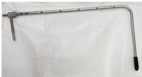
Figure 2 Dwyer pitot tube used as TS.
