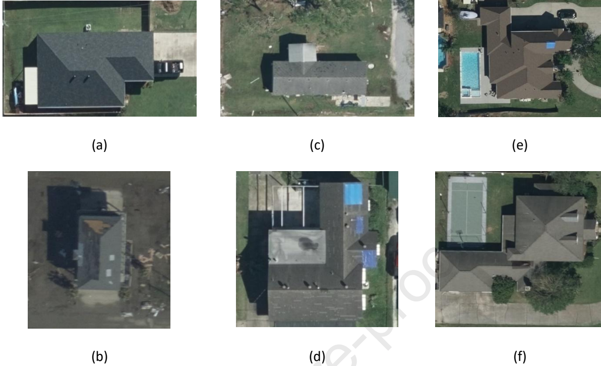
Figure 4. Examples of each roof shape. (a) and (b) are hip roofs, (c) and (d) are gable roofs, and (e) and (f) are complex roofs.
