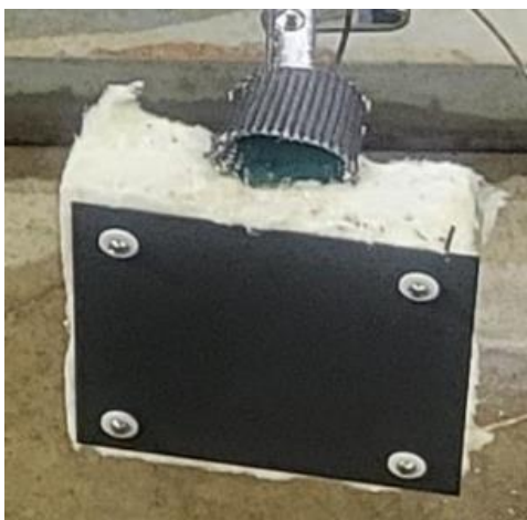
Figure 3. A photo of the front of the 10 cm x 10 cm modified plate thermometer.
