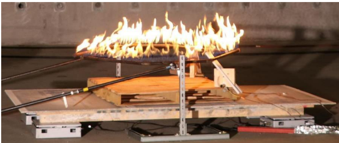
Figure 9. An early version of the burner with flames.
