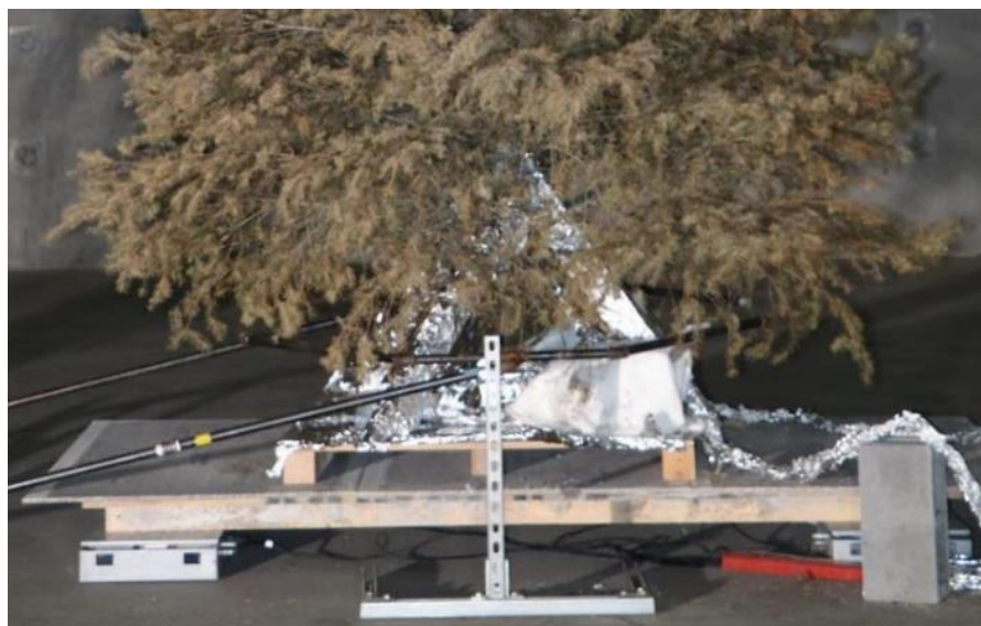
Figure 6. A photograph of the tree stand on the load cell platform.
