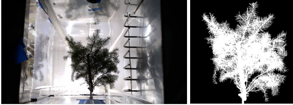
Figure 5: Example of in-situ frontal area measurement for a Douglas fir branch. (left) Single frame from video. (right) Binary image corrected for perspective distortion.
