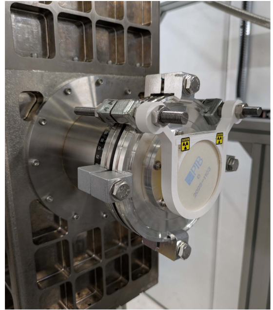
Fig. 5. Radioactive calibration source attached to the end of the TES spectrometer. The source itself consists of radioactive material distributed on a plastic film, labeled with "PTB" in blue text. The plastic film is mounted in a 3D-printed white plastic holder. In normal operation with the antiproton beam, the calibration source will be between the aluminum window on the face of the TES spectrometer and the titanium window on the target chamber to provide continuous calibration data.
