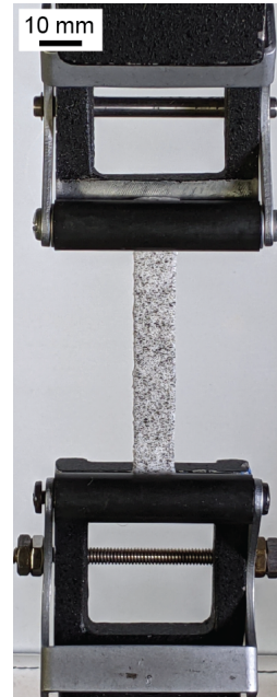
Fig. 1: Snapshot of a speckled specimen mounted in spring loaded grips during a uniaxial test
