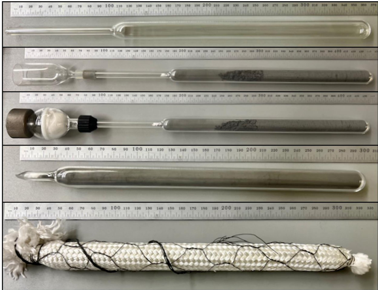
Fig. 6 Ampules at different stages of preparation. Top to bottom: empty ampule, with filling funnel, with adaptor for vacuum system including silica wool filter, sealed ampule (white at the top of the glass is additional silica wool filter in ampule stem), ampule in silica fiber and stainless-steel wrapping.
