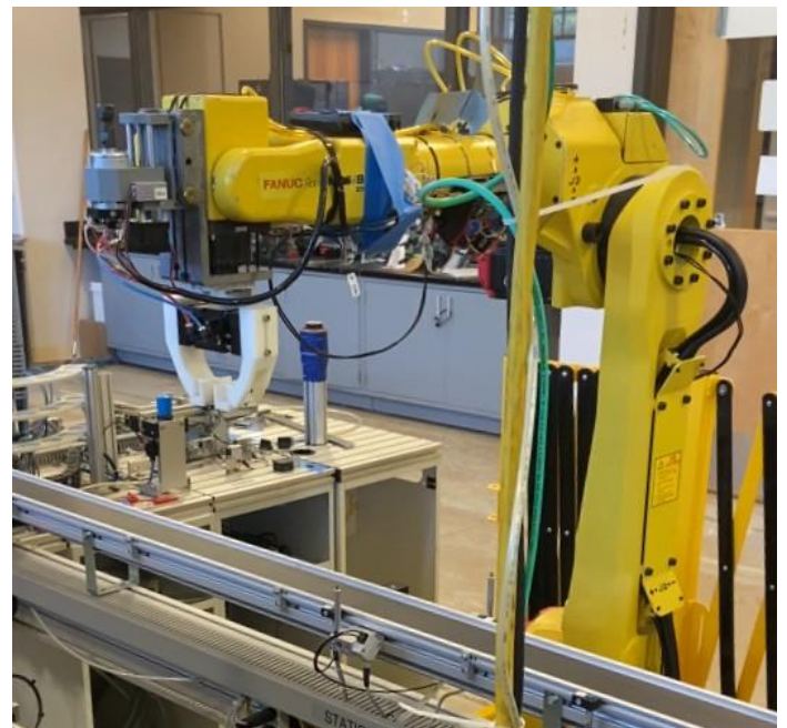
FIGURE 3: Multi-functional FANUC robotic arm with pneumatic parallel jaw gripper and drill tooling.
