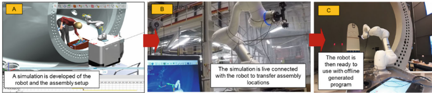
Fig. 12 DT-supported deployment of a robot assistant in wind turbine manufacturing
