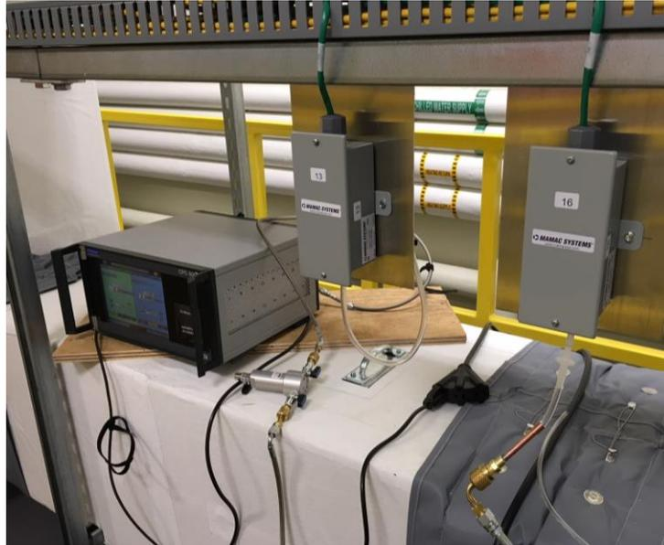
**Fig. 14. Picture of the air pressure calibration setup. The precision pressure controller is at the far left and two pressure transducers (the gray boxes) are visible.**
