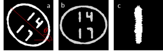
Fig. 4: (a) Microscope image of ellipse with number pattern, (b) rotated ellipse, and (c) isolated number from upper left hand ellipse corner.
