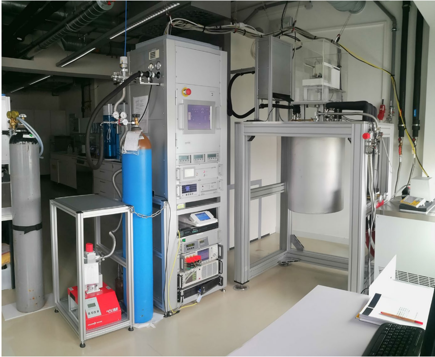
Fig. 1 Photograph of the apparatus. The key components from left to right are: vacuum pumps rack; gas cylinder; instruments and gas dosing system rack; core of the apparatus with the linear motors cage and the analytical balance at the top, and the insulation cylinder containing the measuring cell at the bottom; thermostat bath
