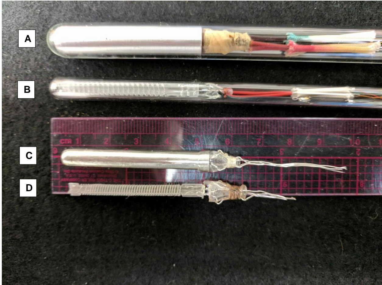
Figure 3. Examples of capsule-type SPRTs as adapted into glass tubing for immersion use in WTP cells. A.) 9.0 mm ID / 11.0 mm OD probe for accommodating traditional capsule-type models. B.) 5.8 mm ID / 7.6 mm OD probe for accommodating low-profile capsule models. C.) traditional-style capsule SPRT with Pt sheath intact. D.) traditional-style capsule SPRT with Pt sheath removed.
