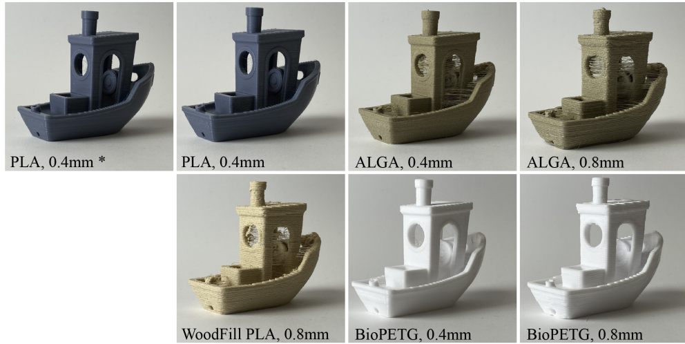
Fig. 6 We deployed our process to produce print parameters for six unique machine, material configurations. We then used those parameters to print the 3DBenchy model [35], a common benchmarking artefact amongst FFF users and researchers. We include here one model printed using heuristically available parameters, which is marked with an asterisk. Our method was able to produce viable print parameters for each filament we tested.
