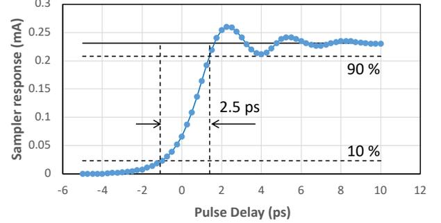
**Fig. 7.** Simulated sampler response of the step-input signal generated by the SQUID DUT shown in Fig. 5.
