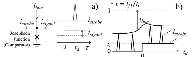
**Fig. 1.** Sampler operation principle indicating the: a) applied currents and b) sampler response obtained for different delays,  $\tau_d$ , between strobe and signal.
