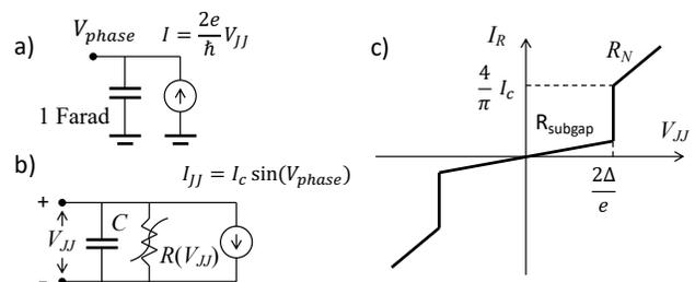
**Fig. 10.** Simplified SPICE model of a Josephson junction consisting of a) an integrator circuit creating a voltage representing the phase of the junction, b) the RCSJ model with a non-linear parallel resistor. c) Piecewise linear current-voltage characteristic of the resistor.
