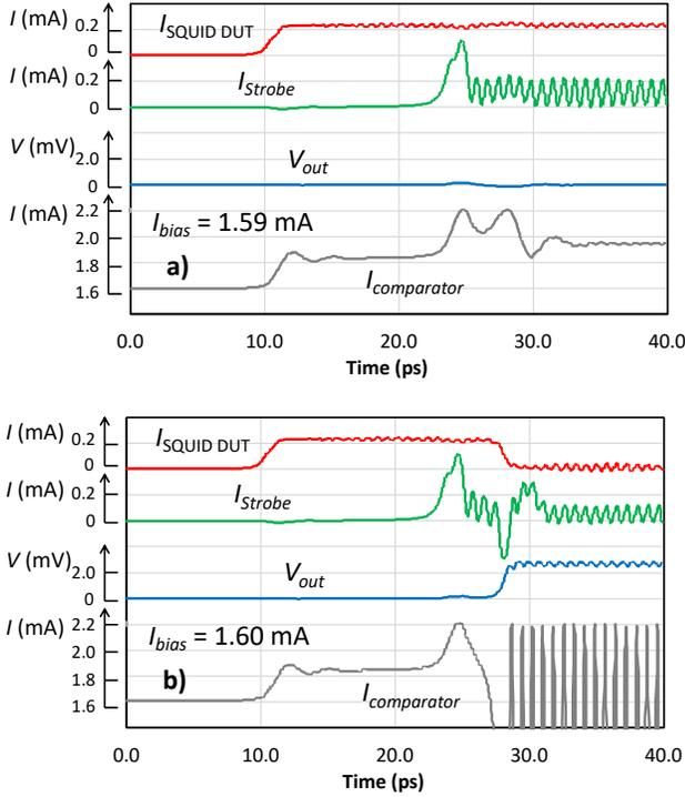
**Fig. 6.** The simulated SQUID DUT current, the strobe current as applied to the comparator, the voltage across the comparator junction, and the Josephson current through the comparator. These were simulated with a comparator bias of a) 1.59 and b) 1.60 mA.
