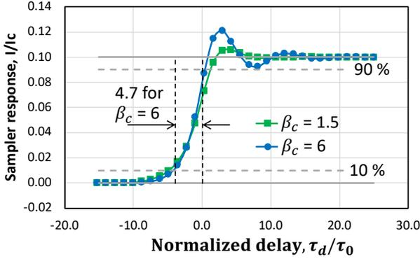
**Fig. 3.** Idealized sampler response for a comparator junction with  $\beta_c = 6$  and 1.5.
