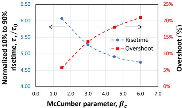
**Fig. 4.** Normalized sampler risetime and overshoot versus the McCumber parameter,  $\beta_c$ .
