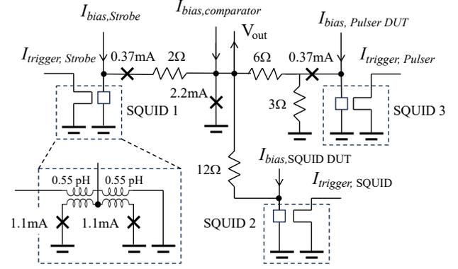
**Fig. 5.** Sampler circuit consisting of a comparator junction, a pulser as a strobe, the SQUID DUT providing a step-input signal and a second pulser with a reduced amplitude as an alternate DUT. The inset shows the detail of SQUIDs 1 through 3 in the circuit.
