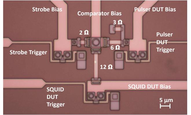
**Fig. 8.** Micrograph of the fabricated sampler circuit including two devices under test (DUT), namely a latching SQUID DUT creating a step-input and a Pulsar DUT creating a pulse.
