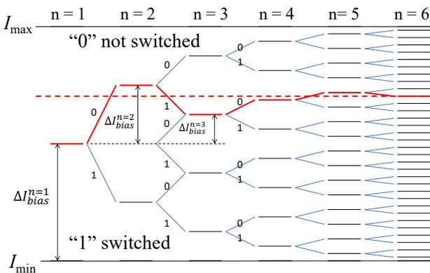
**Fig. 2.** Illustration of the binary search algorithm. See text for detail.
