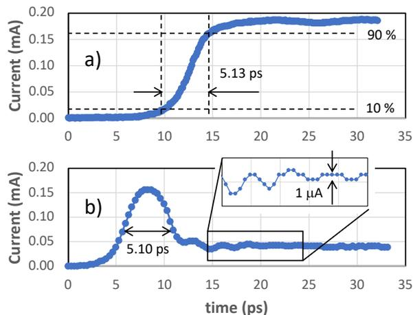
**Fig. 9.** Sampler response measured at 3.6 K of waveforms from a) the latching SQUID DUT and b) the pulser DUT. The inset shows the discretized output with a minimum current step of 1  $\mu\text{A}$ .
