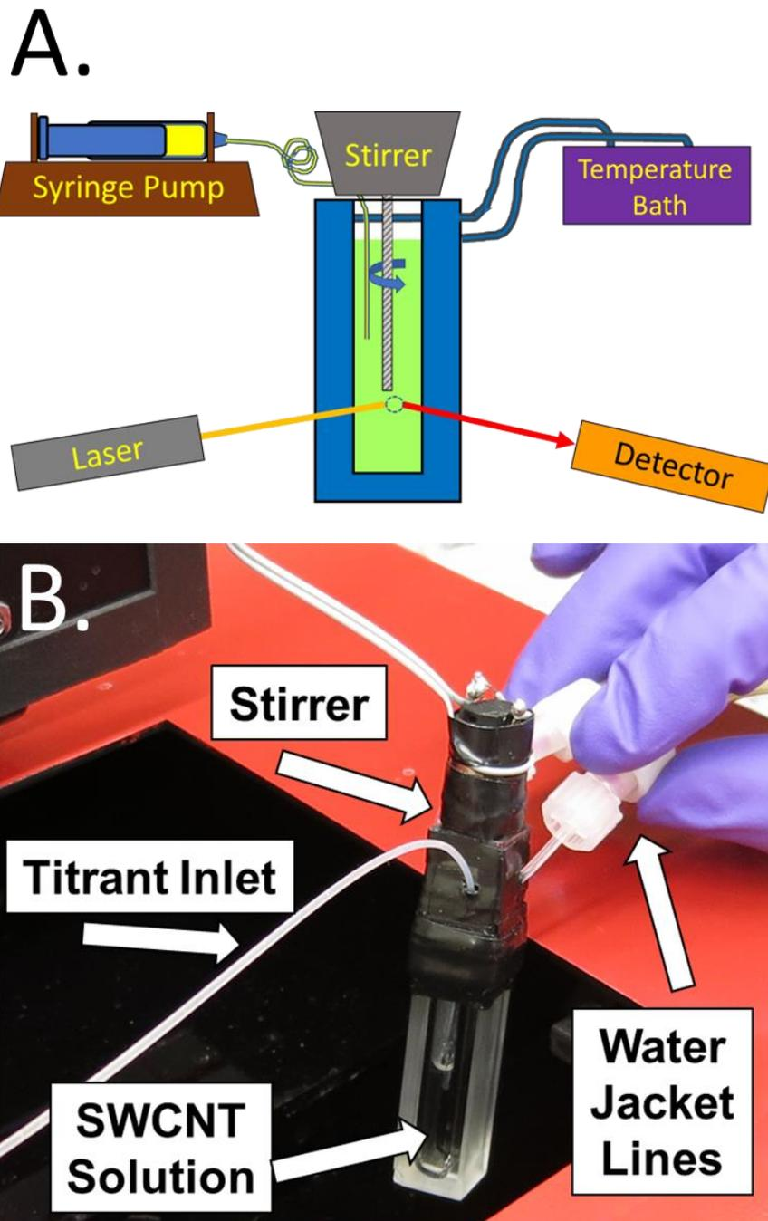
**Figure 1.** A) Schematic of the automated gradient titration setup housed within the fluorescence spectrophotometer. A stirrer provides rapid mixing of the SWCNT solution during titrant addition, while a temperature bath sets and maintains a fixed solution temperature. Fluorescence is measured in a front face collection geometry. B) Photograph of the actual cuvette assembly, with titrant inlet, stirrer, and water jacket temperature control lines noted.
