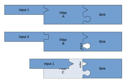
**Fig. 6.** How inputs are chosen for a filter and sink. Input 1 is used with Filter A. Input 2 is used with Filter B. Input 1 is also used with Filter C because Filter C is "nofilter" and Input 1 matches the sink.
