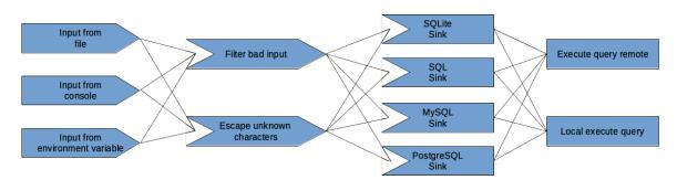
**Fig. 1.** Just three sources of input, two ways of filtering, four sinks, and two query executions yield 48 possible test cases.
