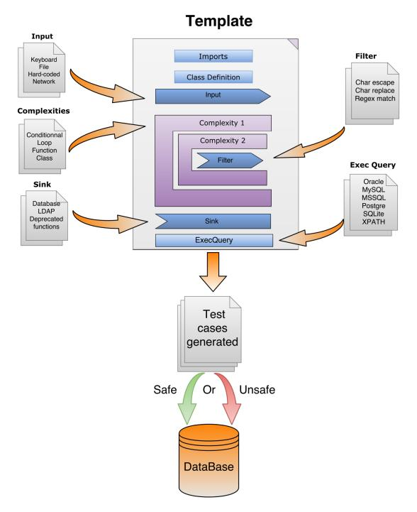
**Fig. 2.** Overview of VTSG test case generation. The File Template specifies how pieces are assembled. Input, Filter, Complexity, Sink, and Execute Query modules provide code. The filter is wrapped with two complexities. An example test case is in Figs. 14 and 15.
