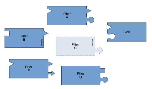
**Fig. 5.** How filters are chosen for a sink. Filters A, B, and C will be used. Filter P is not used because the flaw\_type differs. Filter Q is not used because the output\_type differs.
