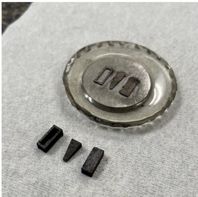
**Fig. 13.** LPBF-built  $\text{Bi}_2\text{Te}_{2.7}\text{Se}_{0.3}$  parts with nonstandard geometries. Prior to part removal, the substrate was mounted in a polymer epoxy to prevent cracks within the substrate from propagating into and breaking the  $\text{Bi}_2\text{Te}_{2.7}\text{Se}_{0.3}$  parts.
