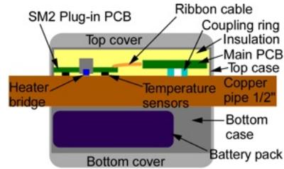
Cross-sectional illustration of packaged sensor module
