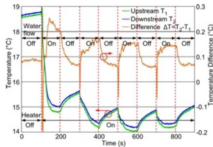
SM2 test results showing  $T_1$  and  $T_2$  readings and  $\Delta T$
