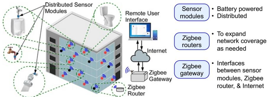
Concept diagram of the wireless sensor network.
