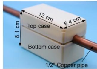
Assembled & packaged sensor module mounted on 1/2" copper pipe
