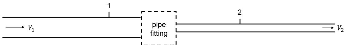
$$\Delta P_{\text{loss}} = (P_1 - P_2) - \Delta P_{\text{friction},1} - \Delta P_{\text{friction},2} - \frac{1}{2} \rho (V_2^2 - V_1^2)$$
