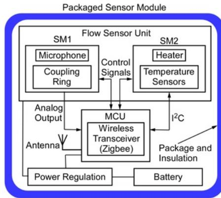
Hardware block diagram of the sensor module.
