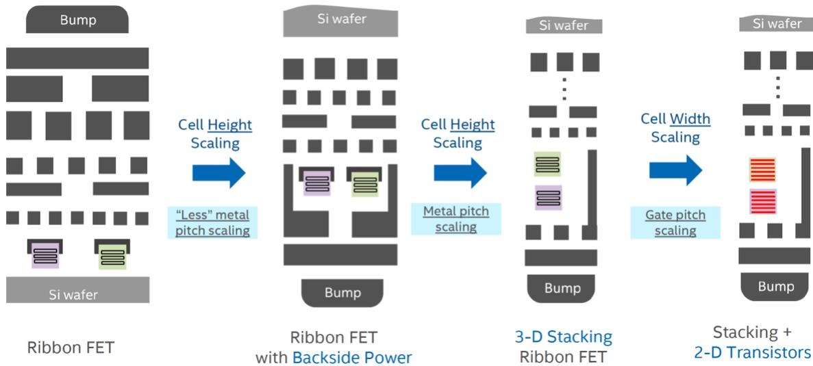
Fig. 8. Example of cell size scaling trends for a ribbon FET where cell width and cell height scaling are needed. Image Credit: Intel, Gstrein *et al.* [54]
