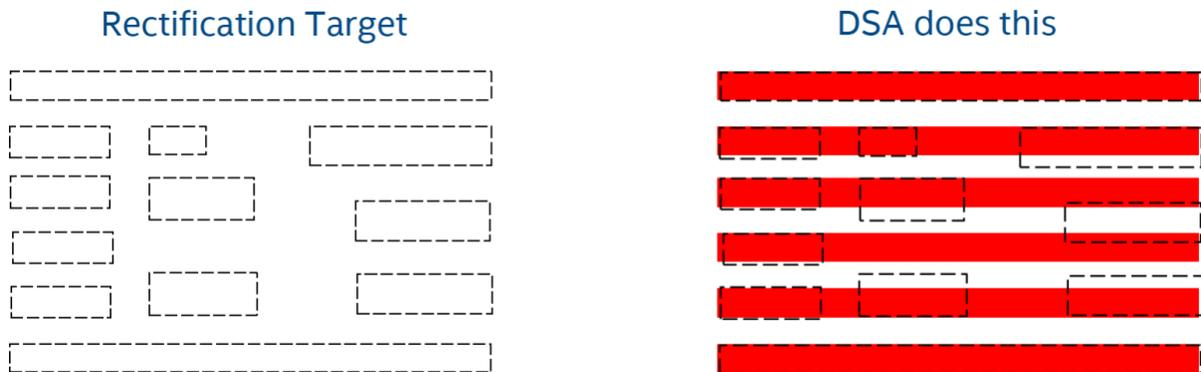
Fig. 11. Diagram showing how DSA does not preserve the target layout, so there is a need for pitch-independent rectification of roughness and defects. Image Credit: Intel
