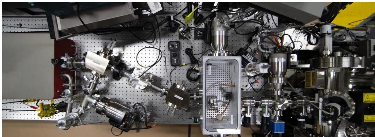
Fig. 18. Atom probe tomography (APT) (top) schematic of the operation (bottom) photograph of the APT located at NIST in Boulder, CO. Image Sources: NIST
