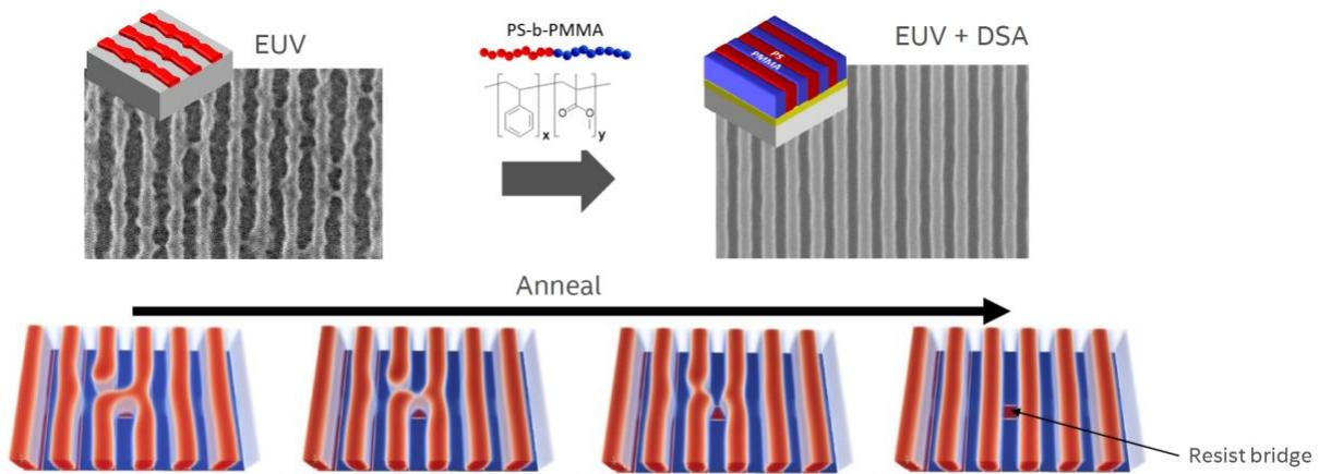
Fig. 9. Example of how using directed self-assembly (DSA) in addition to EUV photoresists improves systematic and random variability. Image Source: Intel
