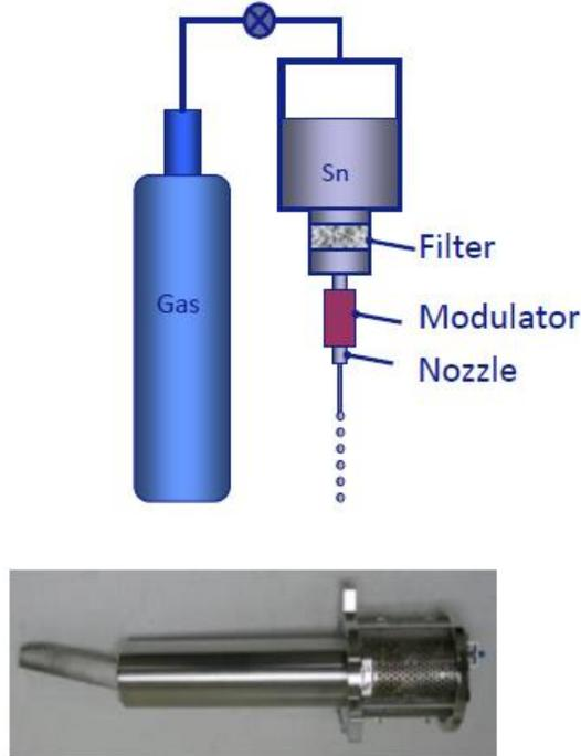
Fig. 3. Schematic (top) and photograph (bottom) of a tin droplet generator. Image Credit: ASML
