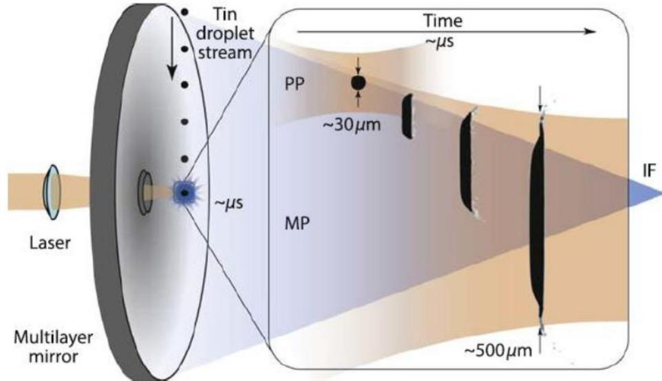
Fig. 12. Diagram showing the concept of EUV collected with near-normal incidence multilayer mirror. Image Credit: Versolanto [46]
