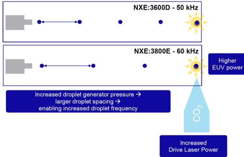
Fig. 5. Schematic in the spatial domain of the droplet generator with different operating pressures to enable higher EUV power. Image Credit: ASML [18]
