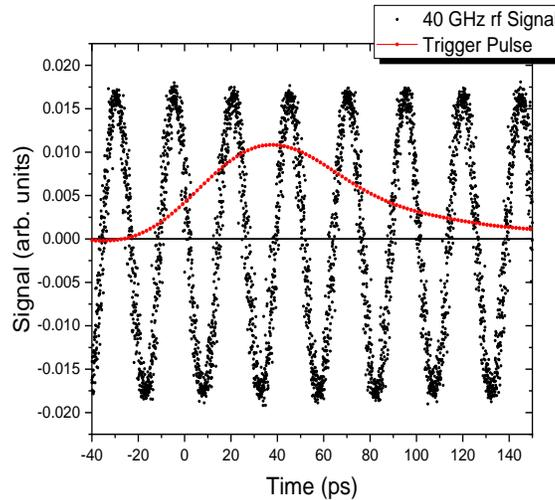
Fig. 15. A 40 GHz signal on a sampling oscilloscope. The trigger pulse (red) came from the pulse used in the HHG system, directly showing the synchronization of the HHG and the 40 GHz signal.
