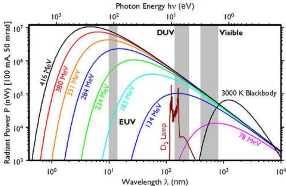
Fig. 17. Synchrotron Radiation Spectrum emitted by SURF at 416 MeV, 380 MeV, 331 MeV, 284 MeV, 234 MeV, 183 MeV, 134 MeV, and 78 MeV in comparison to a 3000 K blackbody and a deuterium lamp.
