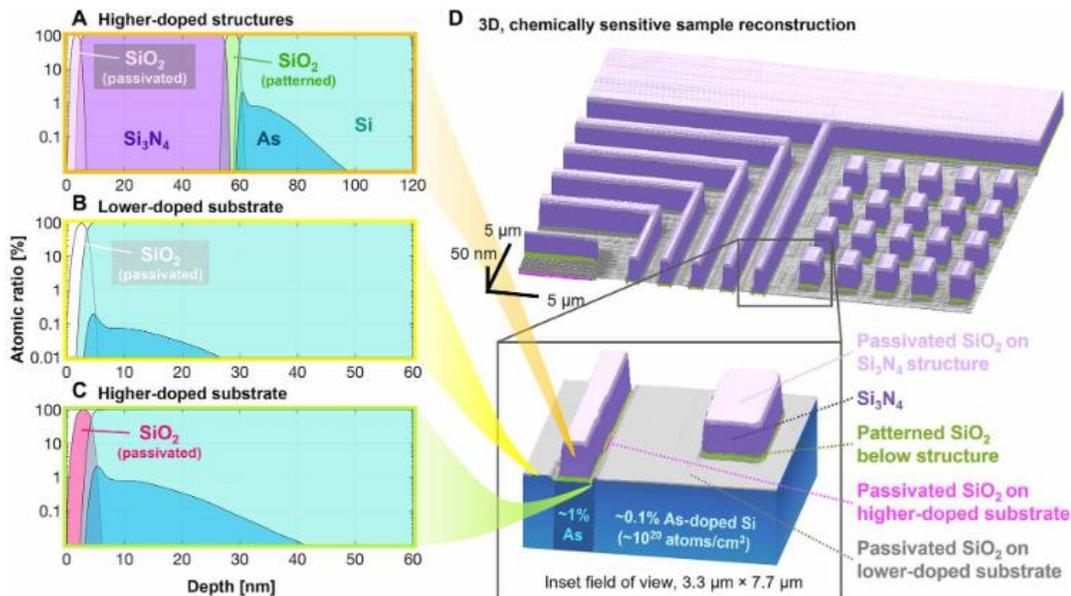
Fig. 16. Example of 3D nanoscale characterization of dopant profiles using a combined reflectometry and ptychography technique. Image from Tanksalvala *et al.* [63]
