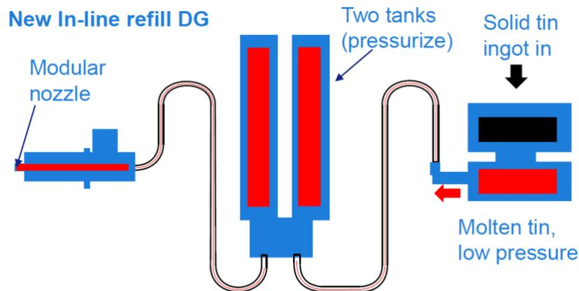
Fig. 4. Schematic of the tin droplet generator with inline refill. Image Credit: Purvis *et al.* [17]
