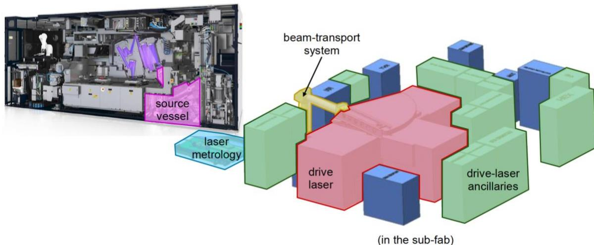
Fig. 2. Graphic of ASML's EUV Lithography source components. Image Credit: ASML
