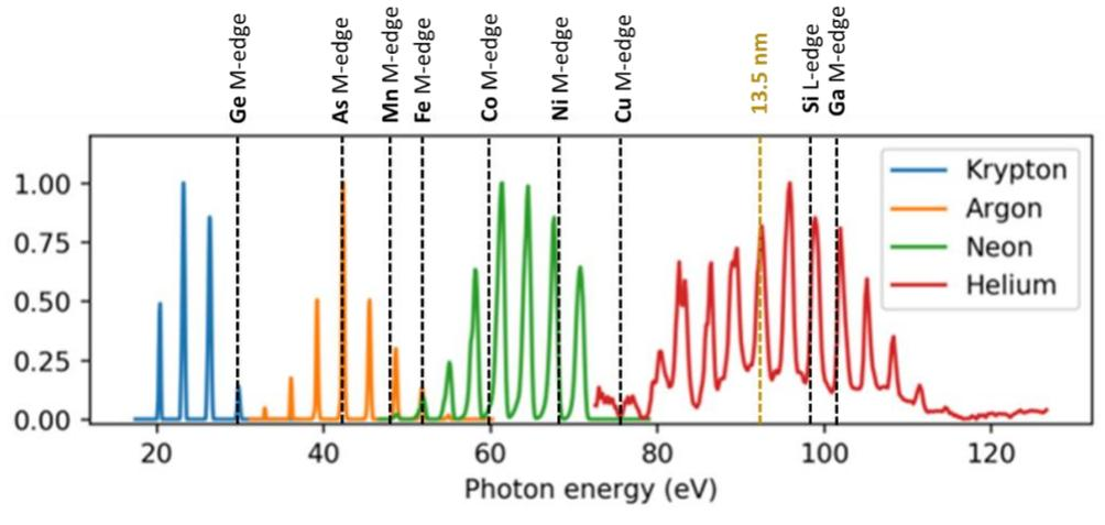
Fig. 13. Output spectrum of the photon energies from the NIST high-harmonic generation source with the location of several atomic core level transitions in relevant materials.
