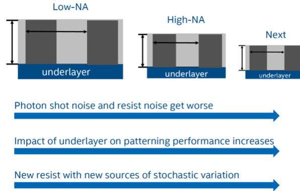
Fig. 10. Diagram showing how new photoresists are needed as the numerical aperture (NA) in EUVL manufacturing transitions from Low-NA to High-NA, and beyond. Image Credit: Intel
