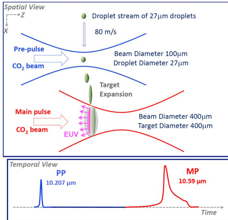
Fig. 7. Diagram showing (top) spatial view and (bottom) temporal view of the two-pulse system to produce EUV light in the semiconductor manufacturing process. Image Source: ASML
