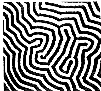
FIG. 1. Stripe domain pattern in film 2 revealed by Faraday rotation of the up and down domains. The stripes are 12 \mu\text{m} wide. Similar stripes in film 1 are 7 \mu\text{m} wide.
