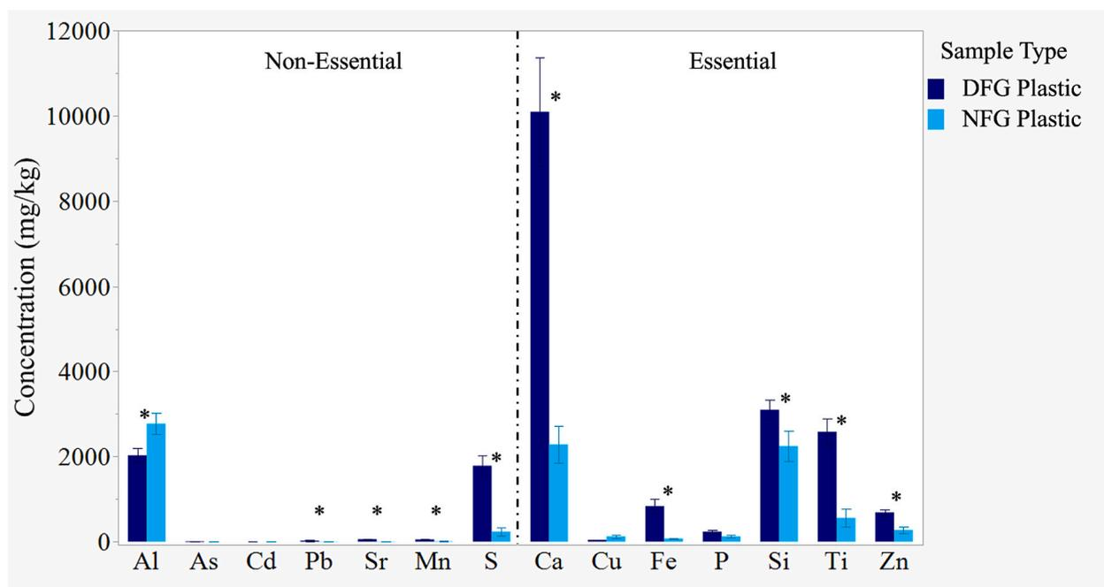
Fig. 8. Elemental concentrations (mg/kg) in plastic components of floating derelict fishing gear (DFG) removed from waters or shorelines near the Hawaiian Islands compared to new/unused fishing gear samples (NFG). Elements are categorized based on whether they are essential for life; the non-essential elements may be considered more toxic. \*Denotes significant differences between DFG and NFG concentrations using R NADA cendiff ( $p < 0.05$ ).
