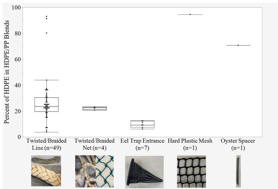
**Fig. 7.** The percentage of HDPE in individual fishing gear samples or components that were identified as a blend of HDPE/PP. Samples were from floating derelict fishing gear removed from nearshore waters or shorelines of O'ahu.
