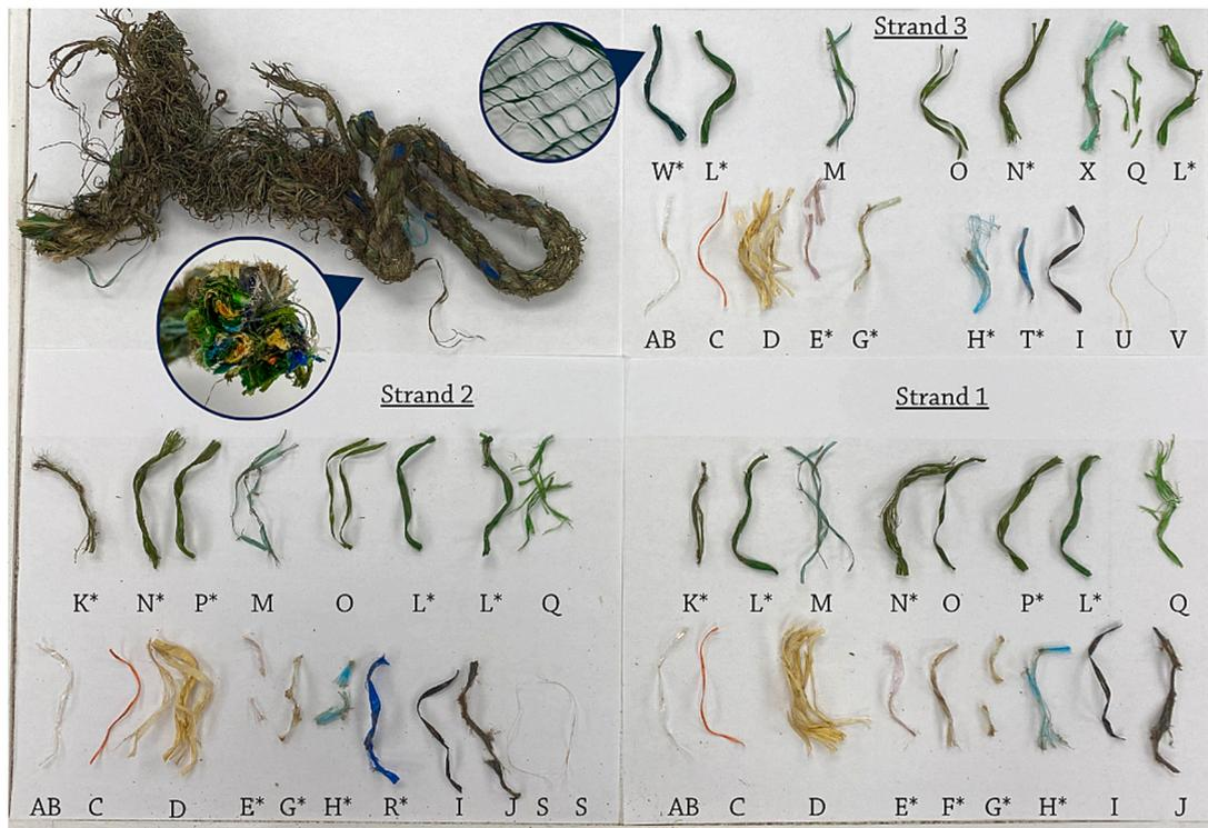
**Fig. 1.** Photograph of the full and cross-section of the case study three-strand twisted line sample (ID OAH\_08\_0290800 in upper left). Individual fibers from each strand were dissected and analyzed. Similar letters represent the same fiber type based on color, opacity, construction, and polymer identification. \*Indicates that the construction type is fibrillated, pictured pulled apart in the top circular image.
