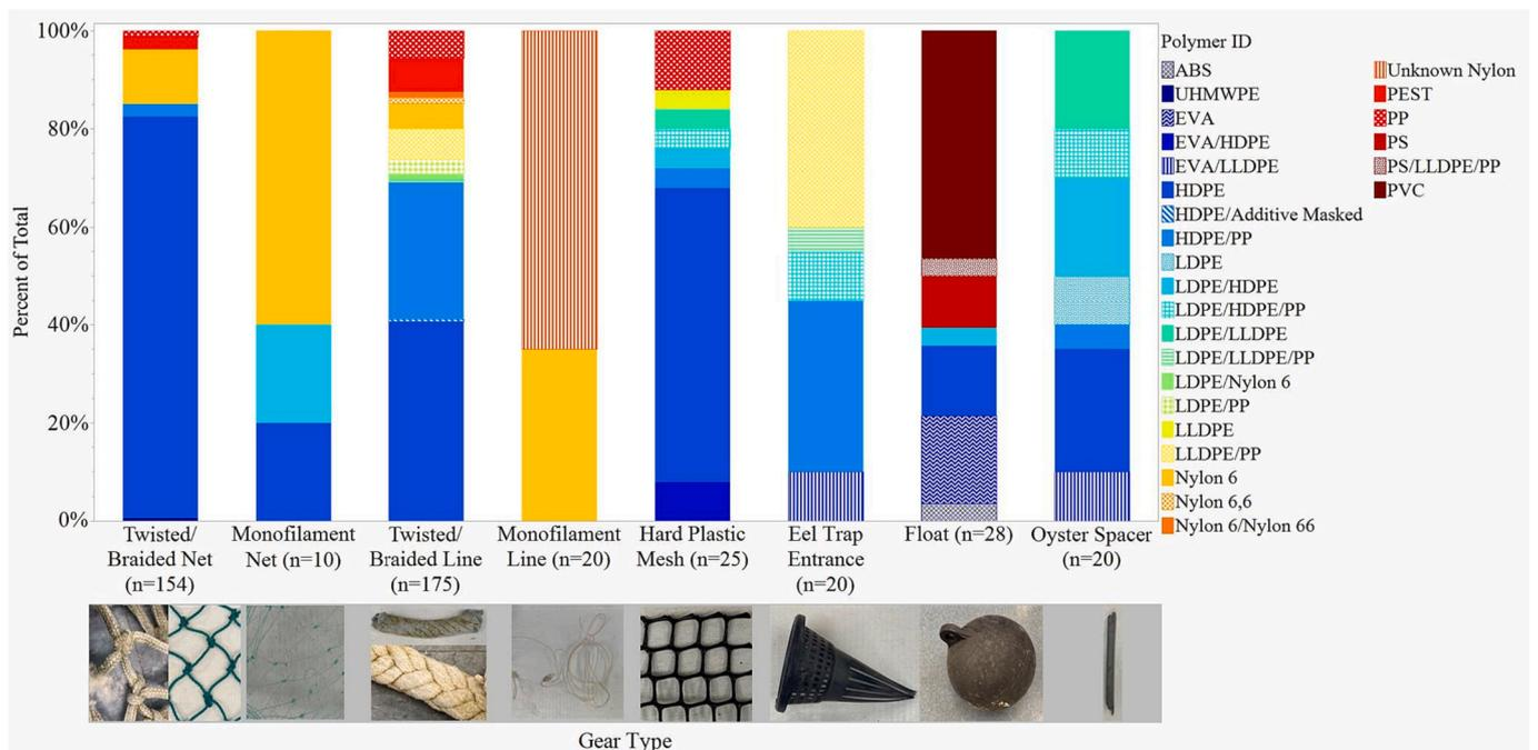
**Fig. 2.** Polymer composition of the eight gear types that were sampled from floating derelict fishing gear removed from nearshore waters or shorelines of O’ahu, Hawai’i. A Fisher exact test revealed significant differences in polymer composition among gear types ( $p < 0.001$ ).
