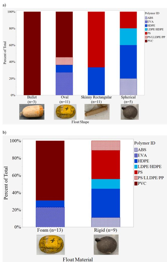
**Fig. 4.** Polymer composition of floats categorized a) into different shapes or b) into foam or rigid plastic forms that were sampled from floating derelict fishing gear removed from nearshore waters or shorelines of O'ahu. Two Fisher exact tests revealed significant differences in polymer composition among float shapes ( $p = 0.01$ ) and again for foam vs. rigid forms ( $p < 0.001$ ).
