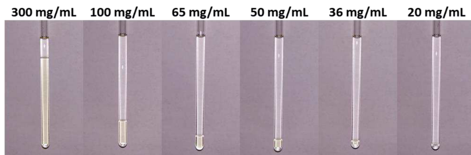
FIG. 2. Photos showing liquid–liquid phase separation of pAPAPS at 12 °C in D 2 O for several concentrations after equilibration at temperature for 24 h.
