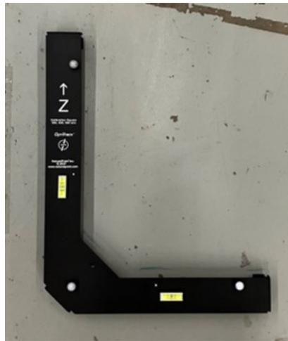
**Fig. 10.** Example of OTS ground-plane placement during calibration.
