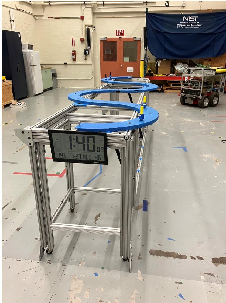
**Fig. 4.** The Type B CMMA used to represent curved, complex parts for mobile manipulator performance measurement.
