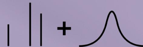
Gaussian detector response convolved with Geant4 energy histogram output
