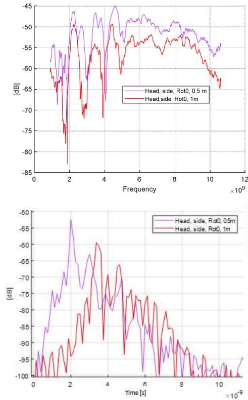
Fig. 5: Off-body channel measurements with the flexible antenna a) Forward transmission coefficient (S21) b) Channel impulse response
