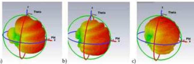
Fig. 2: 3D radiation patterns of the flexible antenna at: (a) 2.45 GHz, (b) 4 GHz, and (c) 5 GHz.
