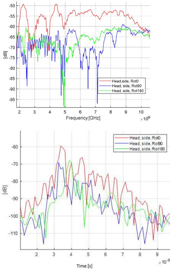
Fig. 6: Impact of body rotation on the channel with flexible antenna a) Forward transmission coefficient (S21) b) Channel impulse response
