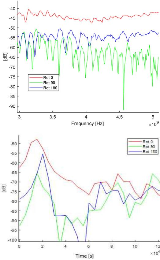
Fig. 8: Impact of body rotation on the channel response with the loop antenna a) Forward transmission coefficient (S21) b) Channel impulse response
