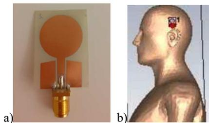
Fig. 1 a) Prototype of flexible antenna, b) simulation model for measuring radiation patterns.
