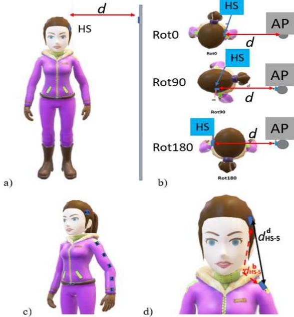
Fig. 4. a) Antenna location on the volunteer's head; b) Off-body measurement scenarios with rotations, c) Antenna locations 1 through 5 for on-body measurement scenarios; and d) LOS and surface distances in the on-body scenario.
