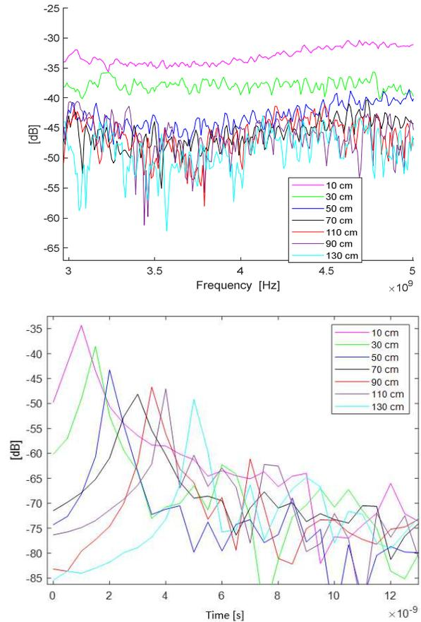
Fig. 7: Off-body channel measurements with the loop antenna a) Forward transmission coefficient (S21) b) Channel impulse response
