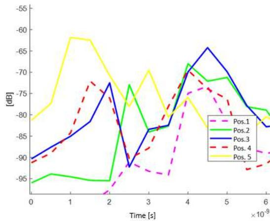
Fig. 10: On-body measurement scenarios with the flexible antenna: a) S21 parameters and b) Channel impulse responses.
