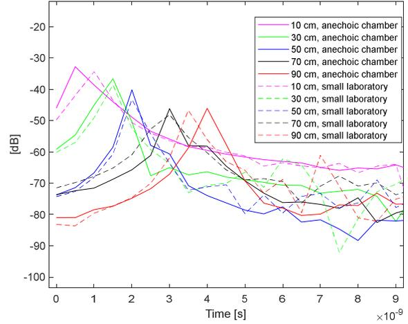
Fig. 9: Comparison of the CIRs obtained from the off-body measurements in the anechoic chamber and the small laboratory.
