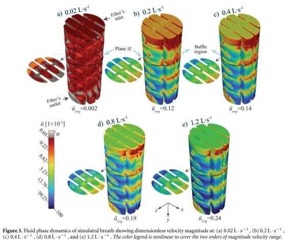
Cut  $\overline{xz}$  plane is y = 8 mm from filter inlet's cross section.
