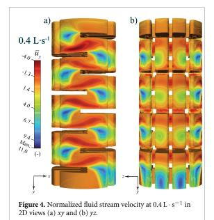
Figure 4 illustrates the normalized fluid stream velocity  $\bar{u}_y$  (along the y axis) developed inside the filter at  $0.4 L \cdot s^{-1}$ , which locally increased up to approximately 11-fold around baffle edges, denoted by blue regions. In contrast, figure 4 also shows that
