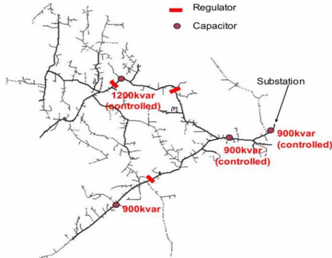
Fig. 1 IEEE 8500 reference grid [18] schematic.
