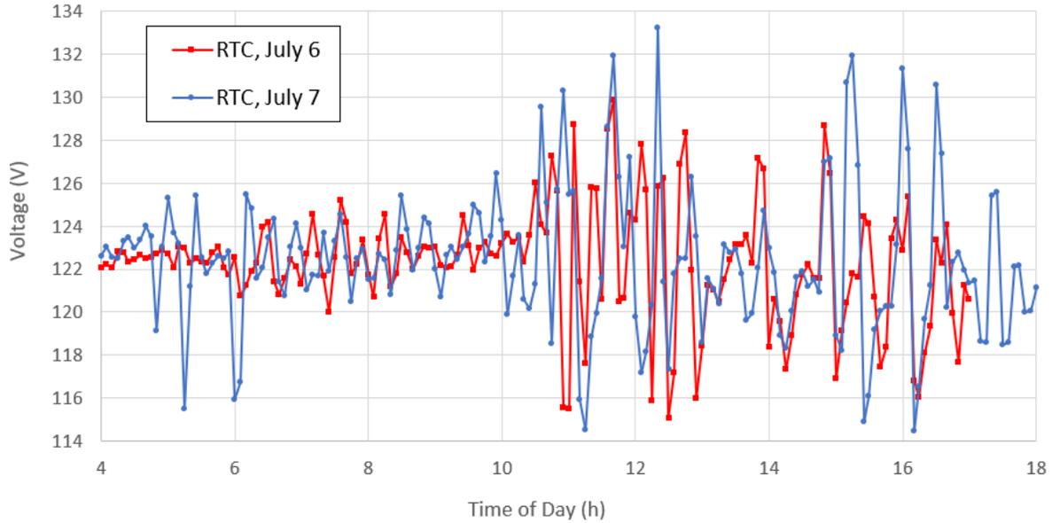
**Fig. 7** Average hourly voltage across house meters, 8500 grid using RTC.
