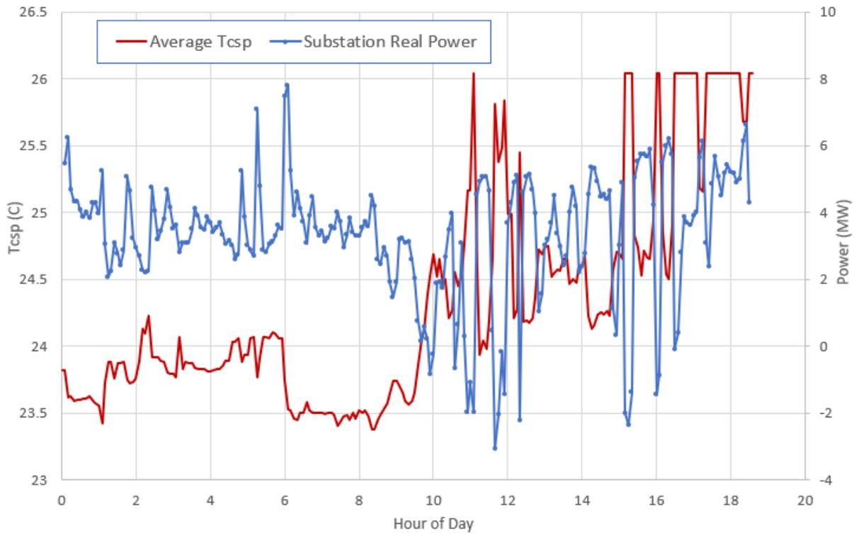
**Fig. 9** RTC average  $T_{csp}$  across all 8500 grid houses compared to the resulting substation real power flow at each 5-min interval, July 7.
