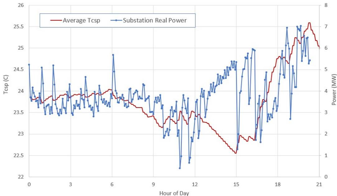
**Fig. 11** LFC average  $T_{csp}$  across all 8500 grid houses together with the resulting substation real power flow at each 5-min interval, July 7.
