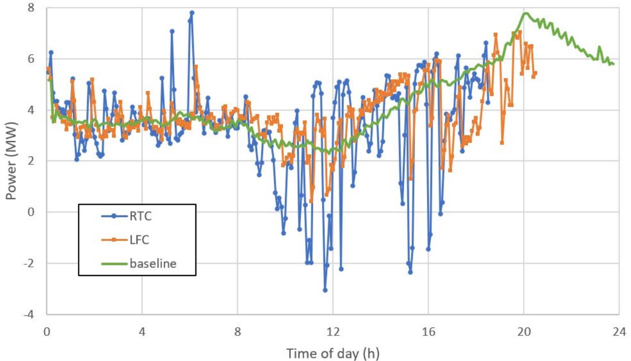
**Fig. 6** Substation real power flow for July 7, comparing baseline (no price response) to RTC and LFC controller adjustment of home temperatures in response to price.
