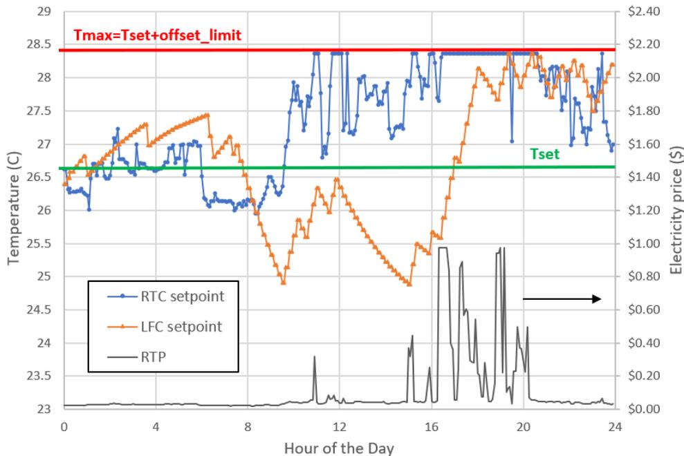
**Fig. 4** Cooling setpoint temperatures from RTC and LFC controllers for a low-comfort house, July 7, 8500 grid. The RTP profile is shown at the bottom.
