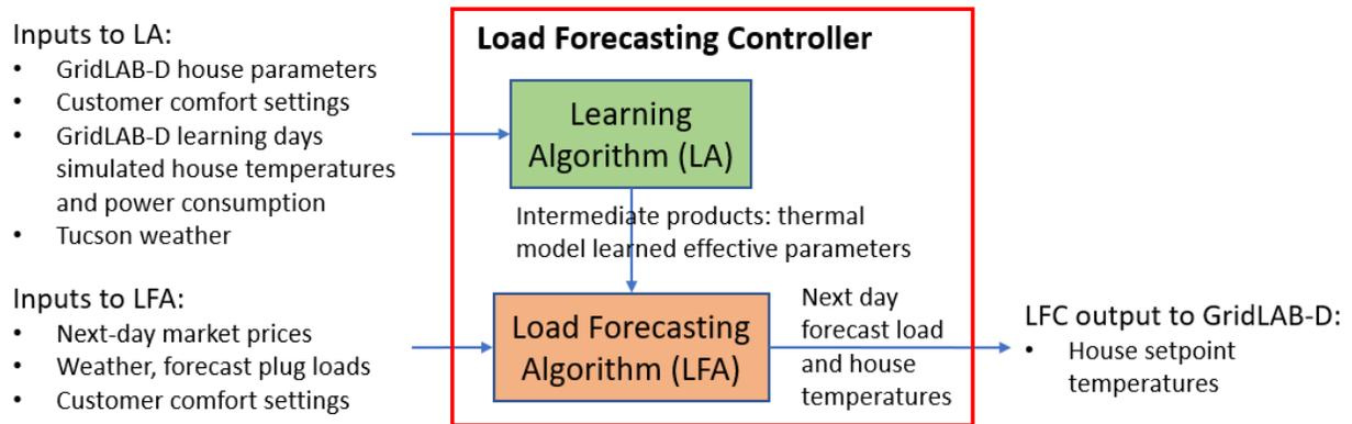
**Fig. 2** Schematic representation of Load Forecasting Controller with information inputs, intermediate products, and outputs to GridLAB-D.
