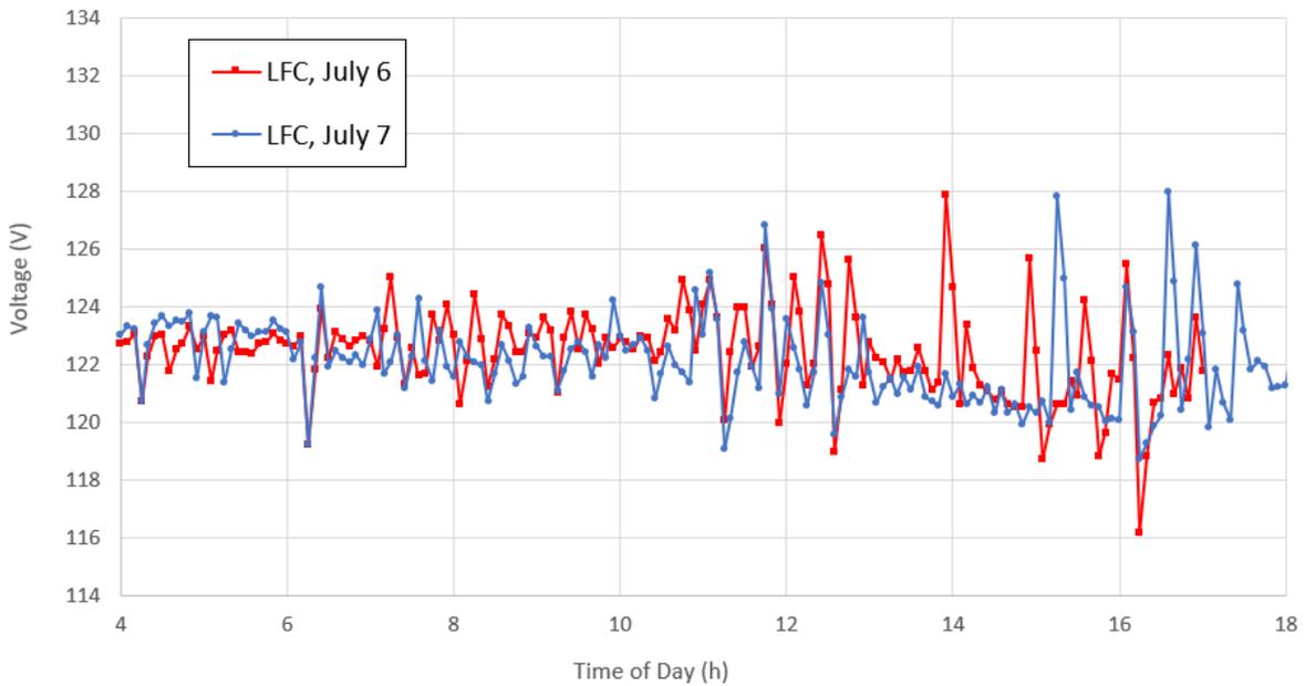
**Fig. 8** Average hourly voltage across house meters, 8500 grid using LFC.
