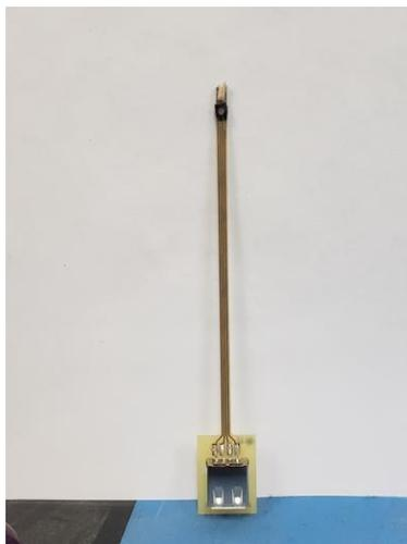
Figure 4. A device mounted to a tee. The tee widths are 4 millimeters with variable lengths.
