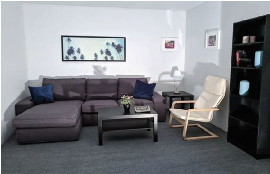
Fig. 12 Picture of furnished compartment test setup under the 10 MW hood at the National Fire Research Laboratory [30]
