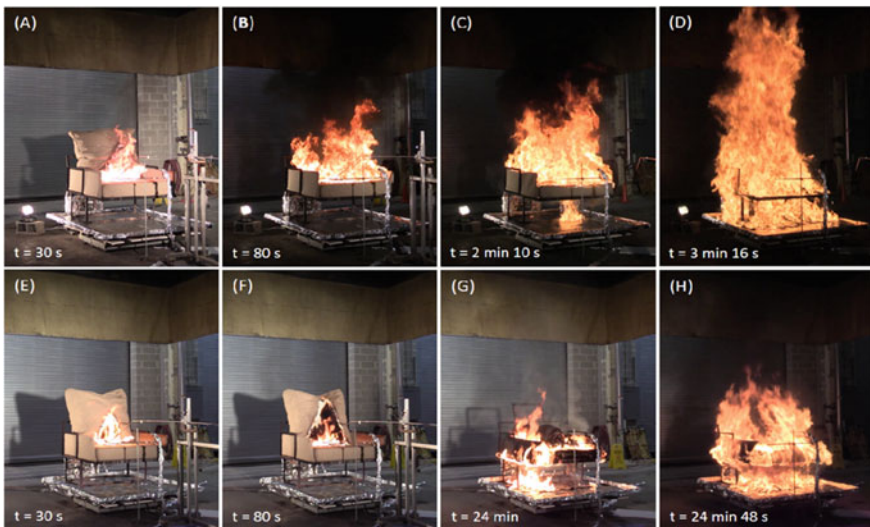
Fig. 7 Snapshots for representative chair mock-ups without a barrier ( a at t = 30 s; b at t = 80 s; c at t = 2 min 10 s; and d at t = 3 min 16 s) and with barrier B6 ( e at t = 30 s; f at t = 80 s; g at t = 24 min; and h at t = 24 min 48 s) [29]
