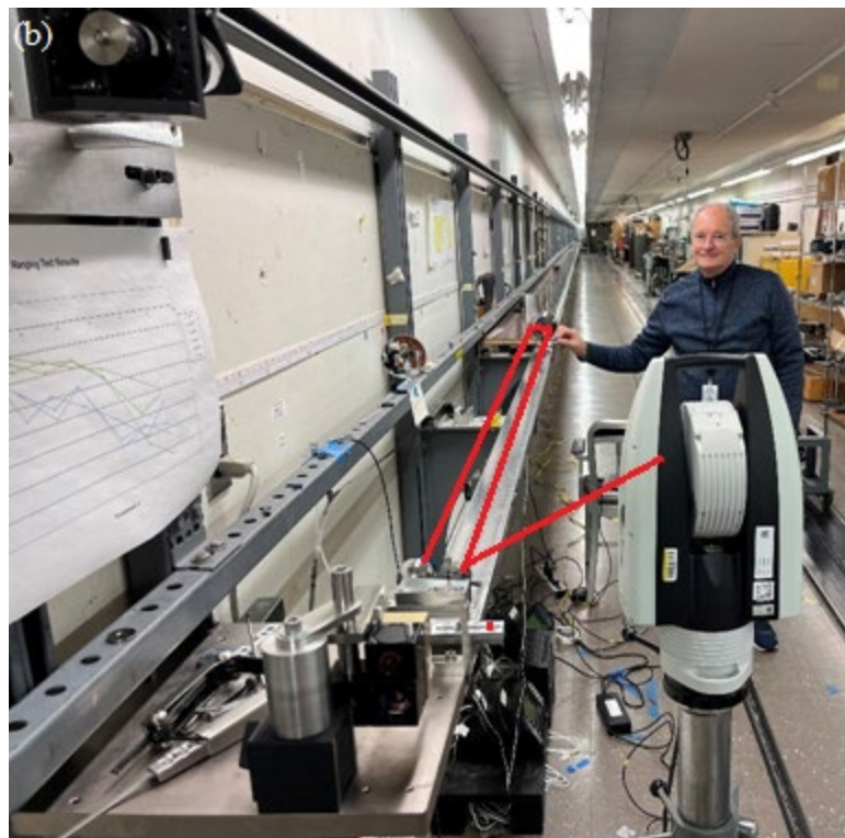
Fig. 12. (a) Fold mirror and SMR placed between the outgoing and incoming reference laser beam of the stand-alone interferometer and (b) the tracker under test placed near the fold mirror and the carriage with one reflector.
