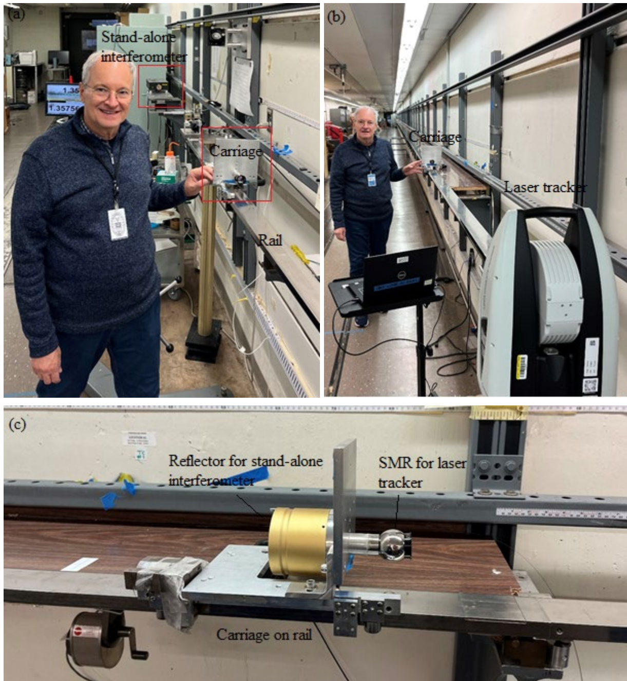
Fig. 2. (a) Stand-alone interferometer and the carriage at one end of the tape tunnel, (b) the tracker under test at the other end of the tape tunnel, (c) the carriage with two reflectors, one for the tracker under test and one for the stand-alone interferometer.
