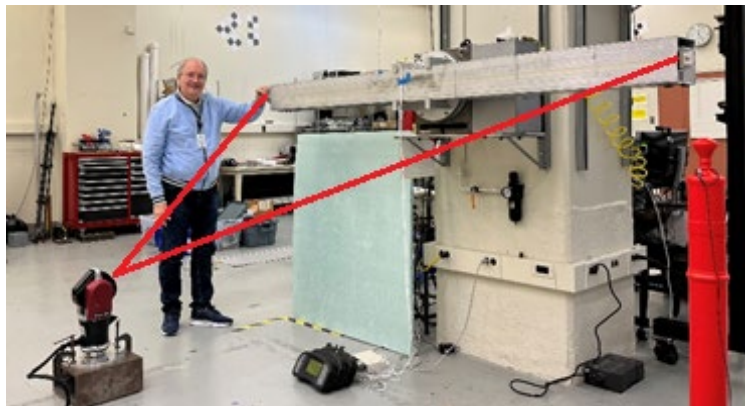
Fig. 9. Two-nest scale bar in raised horizontal position realized by placing the laser tracker on the floor.
