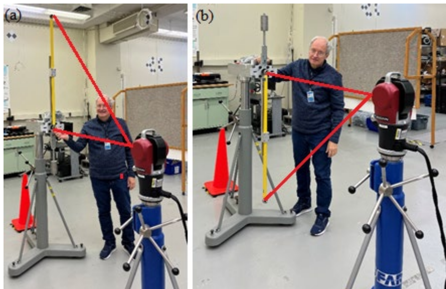
Fig. 14. Half-scale bar in the vertical position, (a) top half measurement (b) bottom half measurement.
