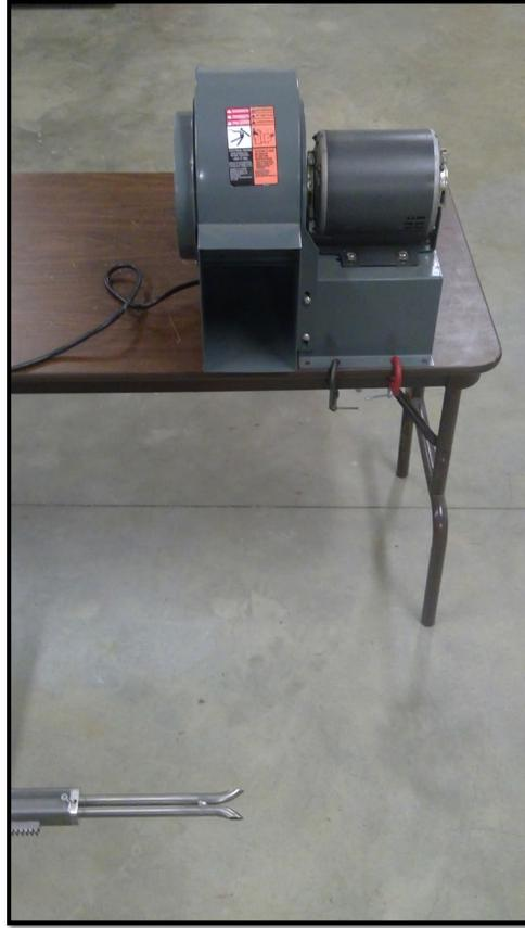
**Fig. 13.** Photograph of electric blower. The blower provided a wind field for testing the yaw-nulling procedure using the S-probe.
