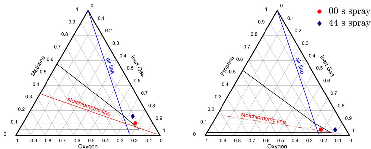
Figure 4: Flammability diagram of gas mixtures surrounding the spark ignitor extracted 10.0 s before the door opened. The 0.0 s and 44.0 s spray times are shown for experiments involving a 37.5 kW methane fire (left) and 25.0 kW propane fire (right) with a fuel flow time of 300 s.
