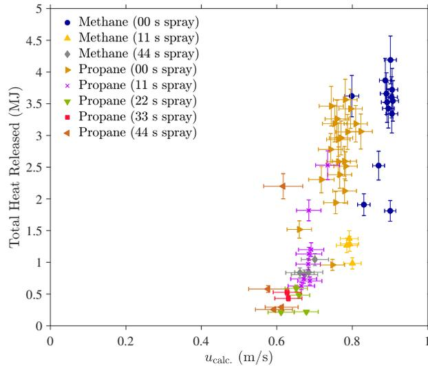
Figure 5: Total heat release of backdrafts plotted as a function of the calculated velocity current. The uncertainty of each measurement was estimated from the law of propagation of uncertainty.
