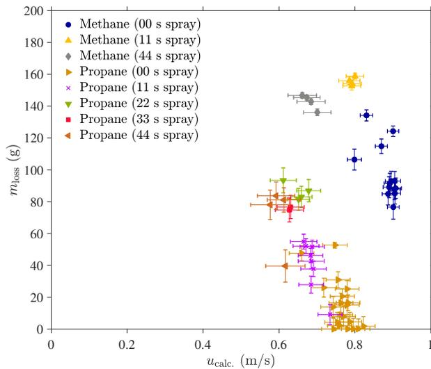
Figure 6: Fuel mass loss plotted as a function of the calculated gravity current velocity. The uncertainty of each measurement was estimated from the law of propagation of uncertainty.
