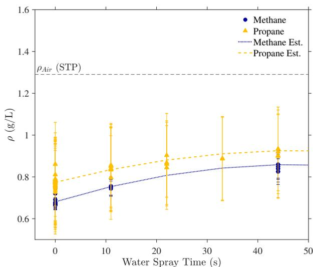
Figure 2: The calculated internal density of the compartment before door opened as a function of water spray time. The uncertainty of the density was estimated from a combination of the Type A and B evaluation of uncertainty.
