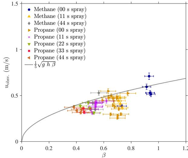
Figure 3: The observed gravity current velocity as a function of the normalized positive density difference. The uncertainty of  $u_{\text{obsv.}}$  was estimated from the Type B evaluation of uncertainty. The uncertainty of  $\beta$  was estimated from the law of propagation of uncertainty.
