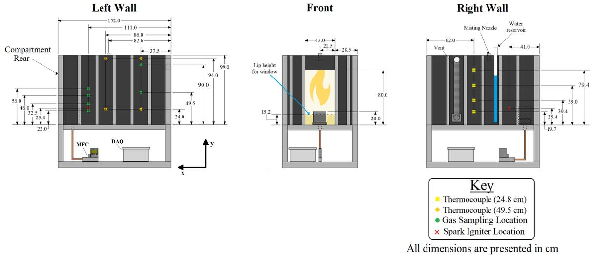
Figure 1: Schematic of the 2/5<sup>th</sup> scale compartment utilized for backdraft experiments. The relative uncertainty of the presented dimensions was estimated to be less than 1%.
